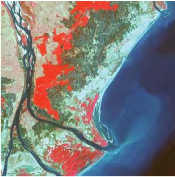
Figure 2.8 False-colour (infrared/red/green) composite IRS1D LISS III image of the Krishna delta on the east coast of India. Coastal features such as beach sand, shoals, mudflats, waterlogged areas and salt affected regions inclusive of salt pans, marsh land, cropland, mangroves and suspended sediments are all clearly discernible. LISS-3 (Section 2.3.5) is a four band (0.52–0.59, 0.62–0.68, 0.77–0.86 and 1.55–1.70 \mu\text{m} ) multispectral sensor that provide 23.5 m resolution coverage. The 23.5 m resolution imagery is resampled to produce a 20 m pixel size. Reproduced with permission from National Remote Sensing Centre of India.
