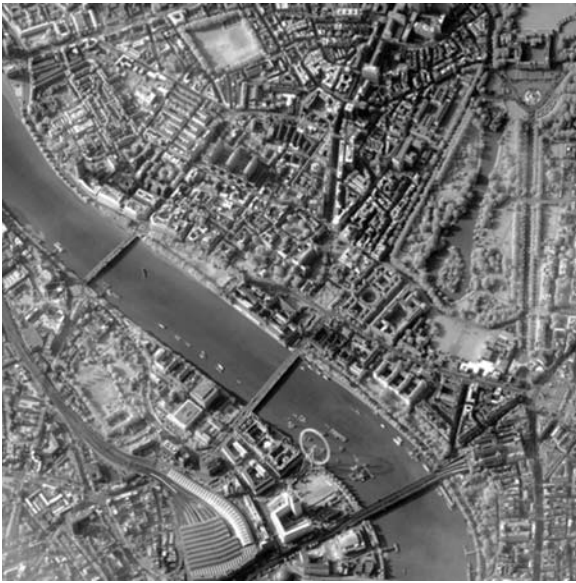
Figure 2.13 IKONOS panchromatic image of central London, showing bridges across the River Thames, the London Eye Ferris wheel (lower centre) and Waterloo railway station (bottom centre). The image has a spatial resolution of 1 m. IKONOS satellite imagery courtesy of GeoEye. Reproduced with permission from DigitalGlobe.
