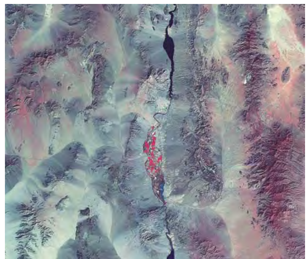
Figure 2.16 Extract from an image acquired by the Algerian AISAT satellite of the Colorado River in Arizona. This is a 1024 \times 1024 pixel ( 33 \times 33 km) extract from the full 600 \times 600 km scene. AISat is a member of SSTL's Disaster Monitoring Constellation (DMC). Reproduced with permission from AISAT-1 Image of the Colorado River (DMC Consortium).
