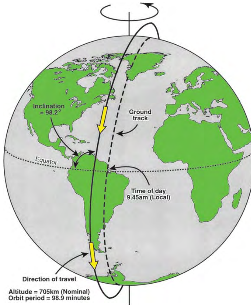
Figure 2.1 Example of a Sun-synchronous orbit. This is the Landsat-4, -5 and -7 orbit, which has an equatorial crossing time of 09.45 (local Sun time) in the descending node. The satellite travels southwards over the illuminated side of the Earth. The Earth rotates through 24.7^\circ during a full satellite orbit. The satellite completes just over 14.5 orbits in a 24-hour period. The Earth is imaged between 82^\circ N and S latitude over a 16-day period. Landsat-7 orbit is similar. Landsat-7 travels about 15 minutes ahead of Terra, which is in the same orbit, so that sensors onboard Terra view the Earth under almost the same conditions as does the Landsat-7 ETM+. Based on Figure 5.1, Landsat 7 Science Data Users Handbook, NASA Goddard Spaceflight Center, Greenbelt, Maryland. http://landsathandbook.gsfc.nasa.gov/handbook/handbook_htmls/chapter5/chapter5.html (accessed 4 January 2009).
