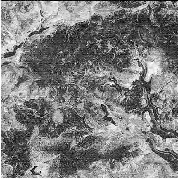
Figure 4.2 Horizontal banding effects can be seen on this Landsat-4 TM band 1 image of part of the High Peak area of Derbyshire, UK. The banding is due to detector imbalance. As there are 16 detectors per band, the horizontal banding pattern repeats every 16th scan line. The image has been contrast-stretched (Section 5.3) in order to emphasise the banding effect. See Section 4.2.2 for more details. Original data courtesy of NASA and USGS.
