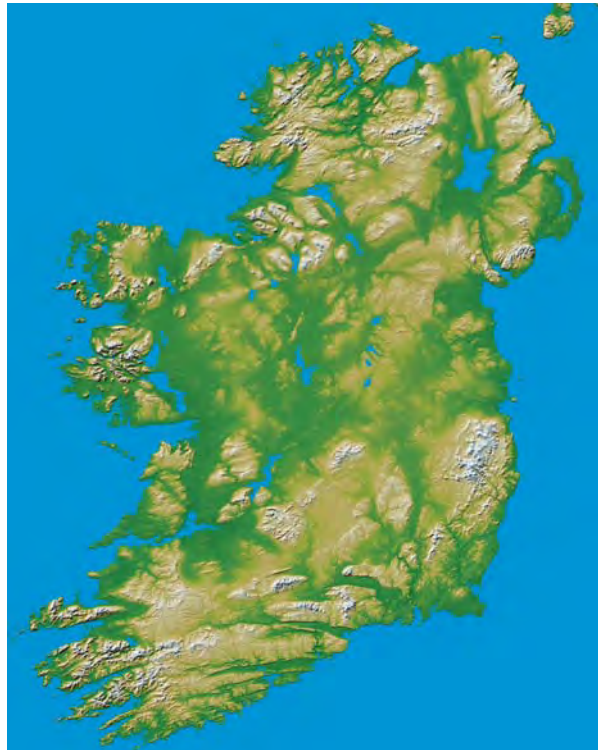
Figure 9.4 Relief map of Ireland from C-band SRTM data. Illumination is from the north-west, so south-east facing slopes are darker. Colour coding (low–high elevations): green–yellow–brown–white. From JPL's Photojournal ( http://photojournal.jpl.nasa.gov/catalog/PIA06672 , accessed 31 July 2009). Courtesy of NASA/JPL/NGA.
