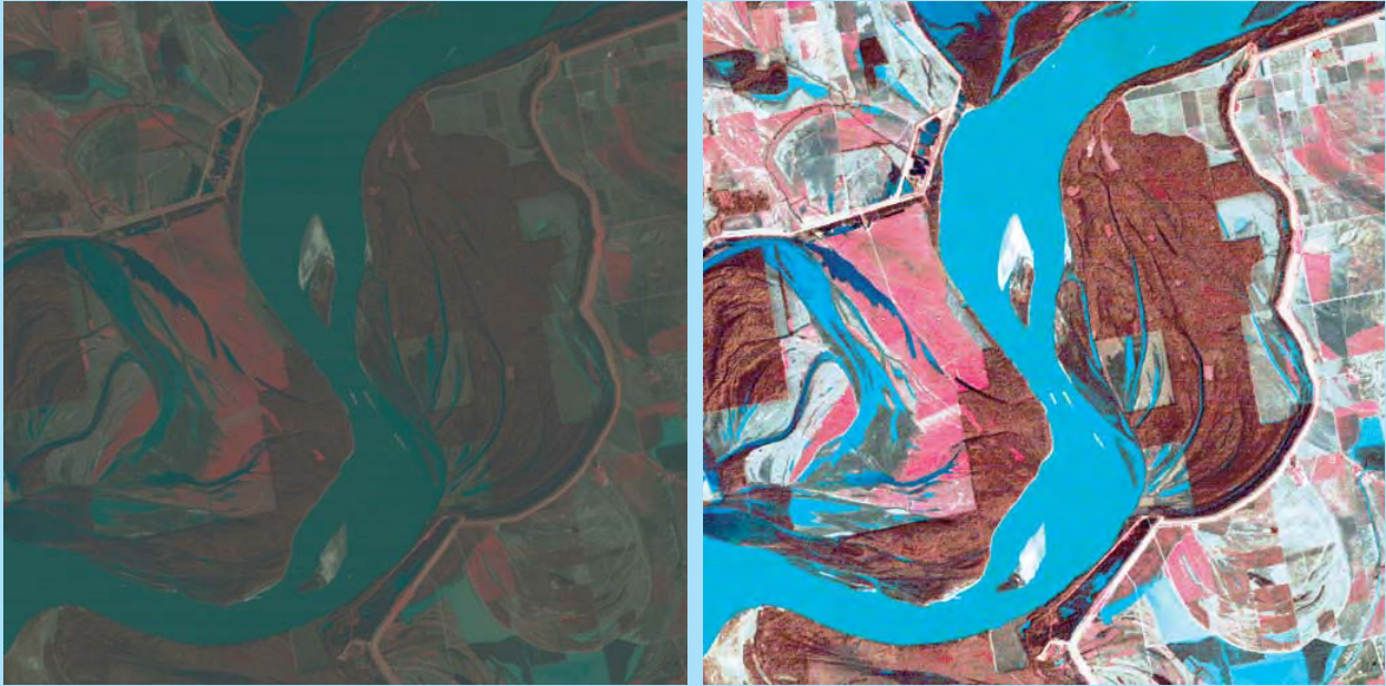
Example 5.1 Figure 7. Contrast stretching can be applied to all three bands of a natural or false colour composite. (a) raw Mississippi image, and (b) after a histogram equalisation contrast stretch.
