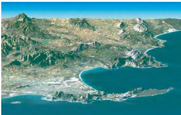
Figure 9.3 Three-dimensional view of Cape Town and the Cape of Good Hope, South Africa. The relief data was obtained from interferometric processing of C-band InSAR data from the SRTM (February 2000) and the colour overlay from Landsat ETM bands 3, 2 and 1 in R, G and B (June, 2000). From JPL's Photojournal ( http://photojournal.jpl.nasa.gov/catalog/PIA04961 , accessed 31 July 2009). Courtesy of NASA/JPL/NIMA.
