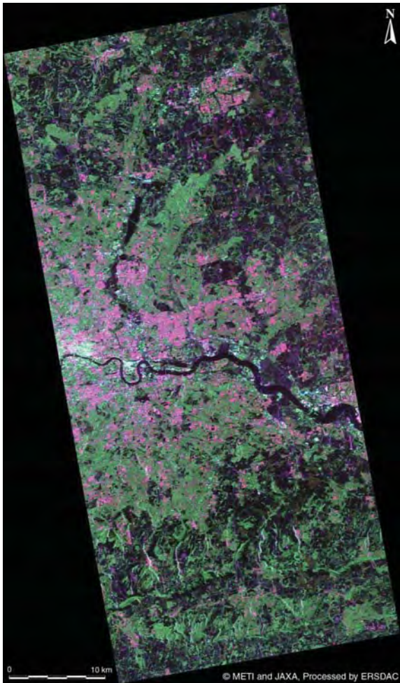
Figure 2.25 ALOS PALSAR image of an area of central/east London captured on 25 April 2007. The red channel is HH polarized, the green is HV and the blue is VV. Research would be needed to determine the meaning of the colours in the image. Source: http://www.palsar.ersdac.or.jp/e/palsarimage/index.html . Image data © METI and JAXA. Processed by ERSDAC.
