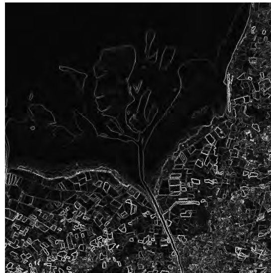
Figure 7.10 (a) Histogram of the image shown in Figure 7.9b. (b) Landsat ETM+ band 4 image of the south-east corner of The Wash in eastern England, after the application of the Roberts Gradient filter and a linear contrast stretch using specified lower and upper limits of 0 and 50 (see the image histogram, (a)). The field boundaries are brought out very clearly, as is the mouth of the River Ouse. One of the challenges of information extraction from images is to derive vector representations of the objects seen in edge-detecting filters such as the Roberts Gradient. Landsat data courtesy NASA/USGS.
