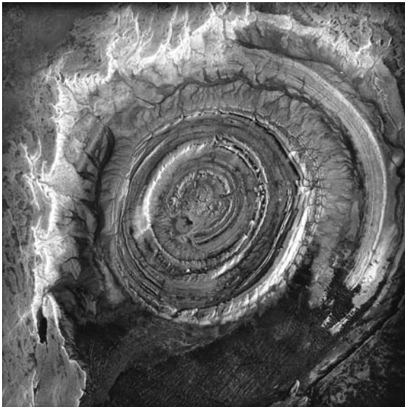
Figure 1.14 X-band Synthetic aperture radar (SAR) image of the Richat geological structure in Mauretania collected by the Italian satellite COSMO-SkyMed 1 on 8 October 2007. The structure is about 60 km in width. COSMO-SkyMed (COntstellatIon of small Satellites for Mediterranean basin Observation) plans to have five satellites in orbit eventually. The third was launched in October, 2008. ( http://www.telespazio.it/GalleryMatera.html ). COSMO-SkyMed Product © ASI-Agencia Spaziale Italiana (YEAR) – All Rights Reserved.
